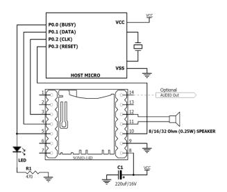
Fig.3. Typical Host Micro Interface
