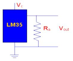
Fig.6 LM 35 with load
