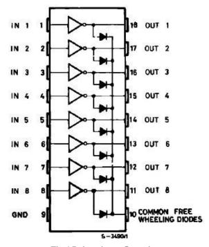
Fig.4 Relay pin configuration
