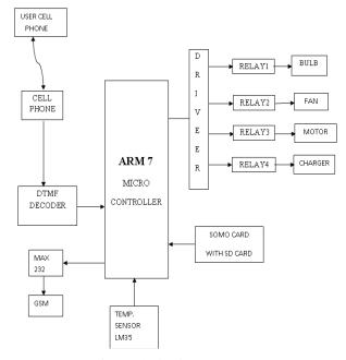
Fig.1. Block Diagram IVRS
